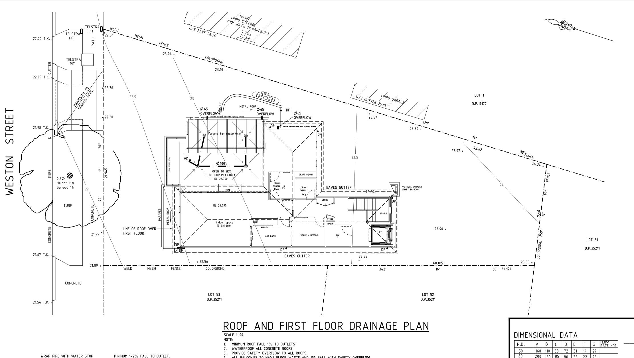
4. ALL BALCONIES TO HAVE FLOOR WASTE AND 1% FALL WITH SAFETY OVERFLOW
